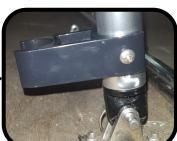
Place the double C clips at the base of the bimini legs and pre-drill with a 9/64" drill bit.
