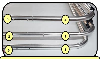
Using the M4 x 30mm bolts from Bag C bolt one end only of the end bow joiners **Parts 6.**
