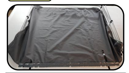
Layout the fabric top as shown and slide the top attachment bars Part 8 into each side of the centre pocket.
