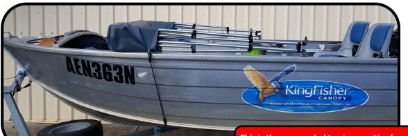
Zip the travel sock onto the closed bimini and lay it over to your preferred traveling position (Bow/Stern) of the boat.
