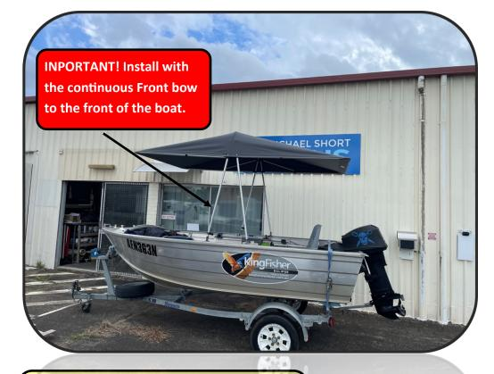
Once you have determined the best position of your Bimini, bolt the deck mounts to your gunnels **500mm** apart using the supplied M5 x 30mm countersunk screws (**Parts bag D**).
