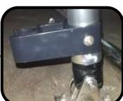
Place the double C clips at the base of the bimini legs and pre-drill with a 9/64" drill bit.
